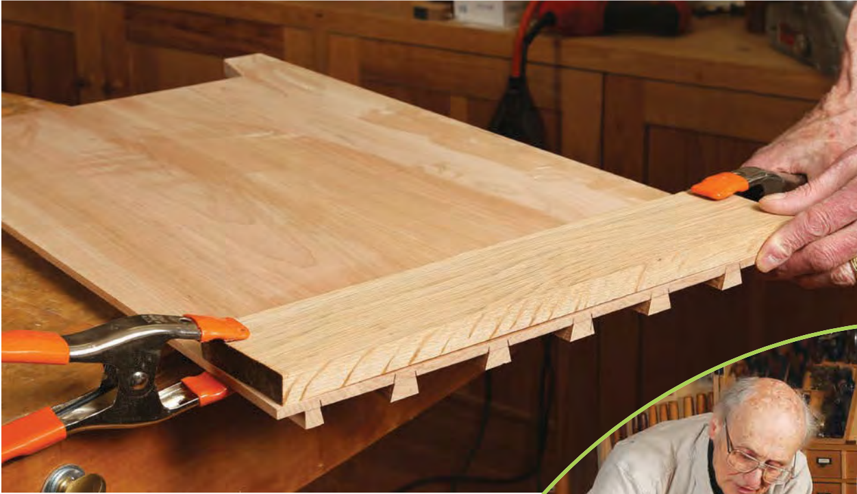
Clamping block does double duty. With spring clamps, attach a block across the dovetails at the top of the sides. This protects the surface of the work while acting as a clamping caul.
