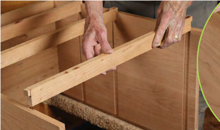
Mark in place. Place the stretchers into the dados. The shoulder-to-shoulder distance of the stretchers should fit nicely between the dados, and the dovetails should overlap the front edge of the case sides. Knife around the dovetails to transfer their location to the sides.
