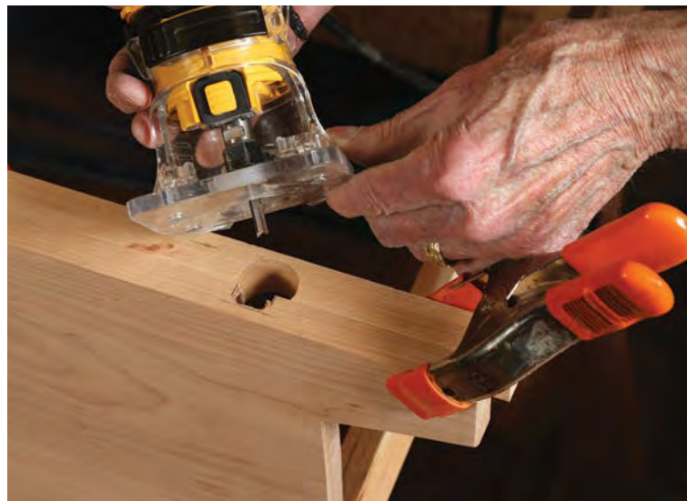
Mark in place. Place the stretchers into the dados. The shoulder-to-shoulder distance of the stretchers should fit nicely between the dados, and the dovetails should overlap the front edge of the case sides. Knife around the dovetails to transfer their location to the sides.
