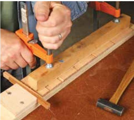
Engage the wedges. Tap the wedges toward each other (top), filling up the extra space between them and the panel pieces. This pushes all the pressure toward the clamped end. Once the pieces are all tight to each other, clamp the other end of the caul to keep the pieces flat while they are drying (above).
