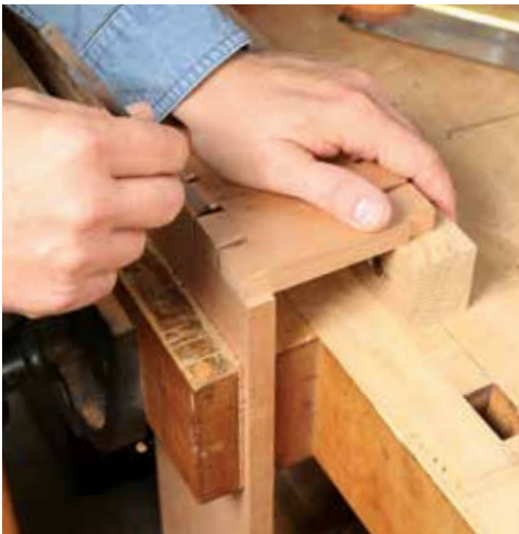
Cut tails and pins. Sterns cuts the tails on the short side pieces first. Then he transfers the layout to the pin boards using the backs as reference to ensure the overhang is at the front. He uses a chopping block as a chisel guide on the shoulder line.
