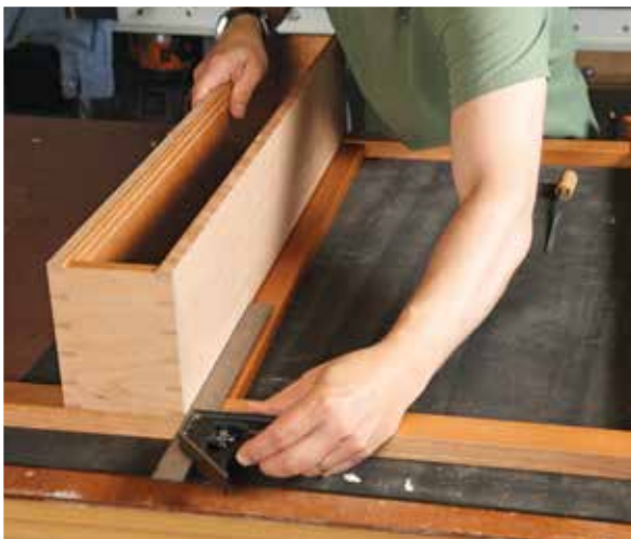
Put the box in its place. Set the box on the mirror frame and mark its location. Using a flush cutting bit (or rub collar) and two fences clamped to the frame, rout the dadoes for the box in the stiles and the bottom \frac{1}{4} in. of the lower rail.
