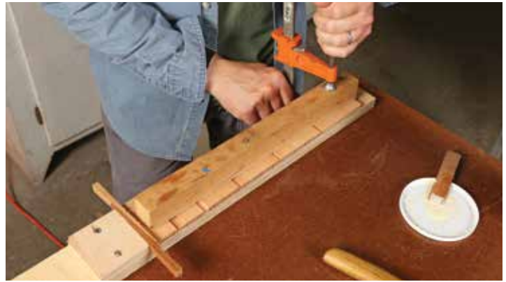
Clamp one end. As you apply glue, assemble all the panel parts and splines on the jig with the two opposing wedges against the stop block (but not yet tightened). Set a caul across the width of the pieces, and apply clamp pressure at the end of the caul farthest from the stop block.
