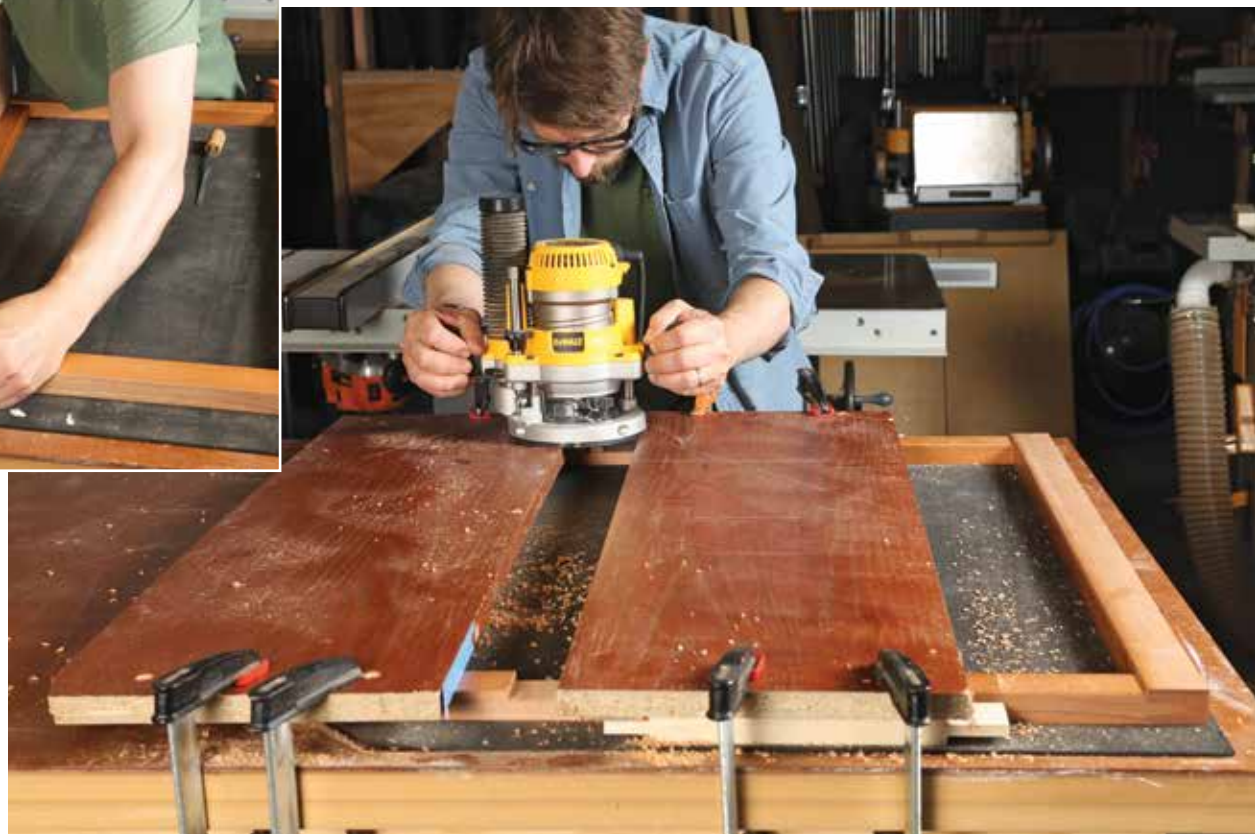
Put the box in its place. Set the box on the mirror frame and mark its location. Using a flush cutting bit (or rub collar) and two fences clamped to the frame, rout the dadoes for the box in the stiles and the bottom \frac{1}{4} in. of the lower rail.
