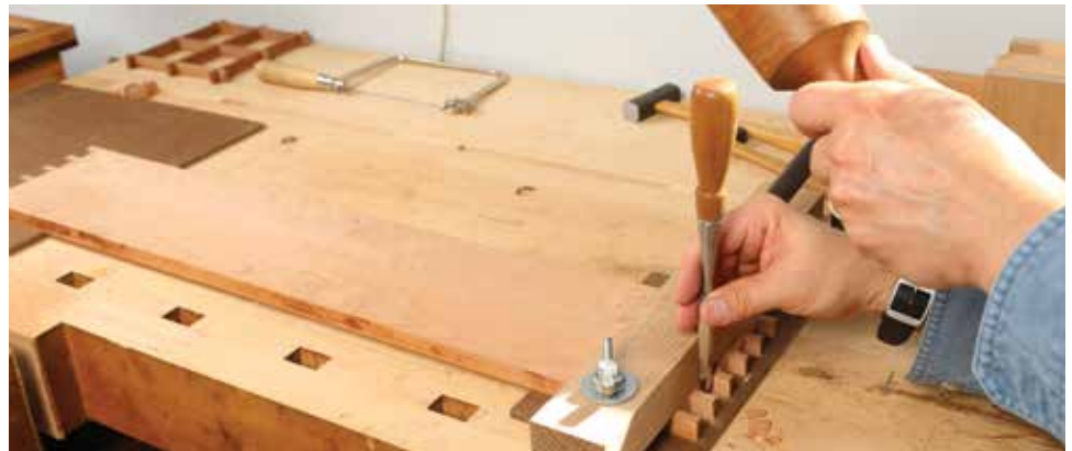
Cut tails and pins. Sterns cuts the tails on the short side pieces first. Then he transfers the layout to the pin boards using the backs as reference to ensure the overhang is at the front. He uses a chopping block as a chisel guide on the shoulder line.
