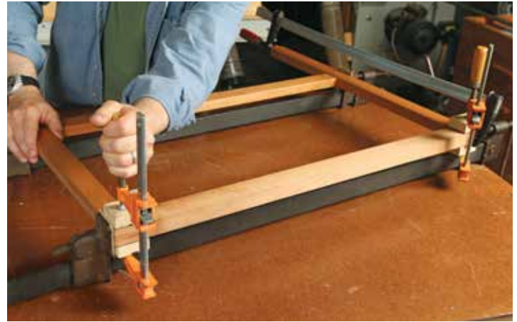
Assemble the mirror frame. Gluing both rails to the stiles at once, Sterns applies pressure across the assembly with bar clamps. But he also squeezes the bridle joints tight with F-clamps.
