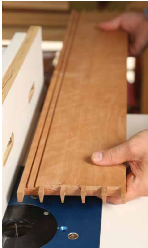
Sliding door infrastructure. At the router table, cut grooves for the sliding doors. The depth of the top groove is slightly greater than the height of the top tongue. The bottom groove equals the bottom door tongue minus the bottom door reveal. Aim for less than a \frac{1}{16} -in. reveal between the door and the case.
