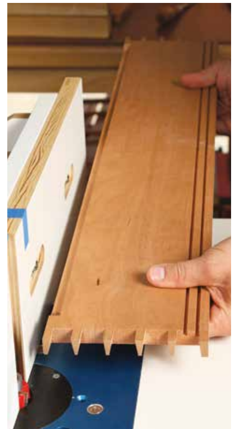
A rabbet for the back panel. Again at the router table, cut the stopped rabbet to hold the frame-and-panel back. Sterns uses blue tape to mark the starting and stopping points on the router fence.
