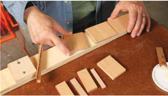
Help from a clamping jig. To simplify assembling the many small panel parts and splines into one wide panel, do the glue-up on a piece of plywood long enough to accommodate all the pieces plus a stop block, two opposing wedges, and a little extra space for the wedges to do their magic.
