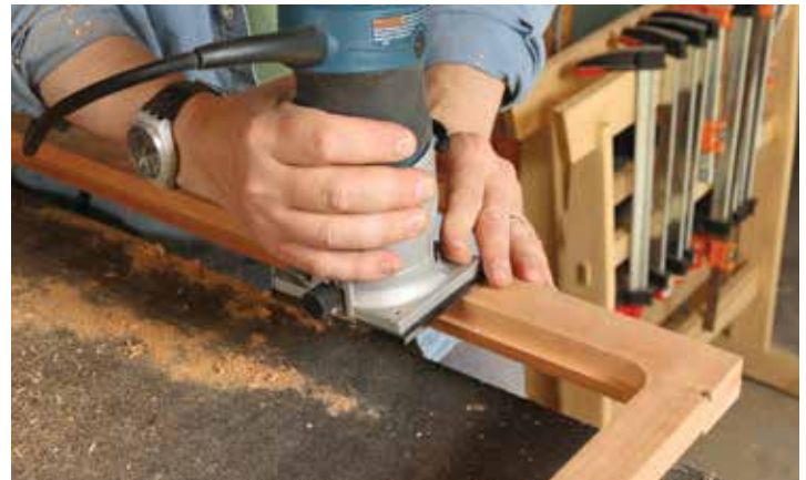
Rabbets for the mirror and French cleat. Once the glue is dry, rout the rabbets for the mirror, plywood backing, and French cleat in the back of the mirror frame. With a chisel, square off all the rounded corners except the top ones for the French cleat, which are left round.
