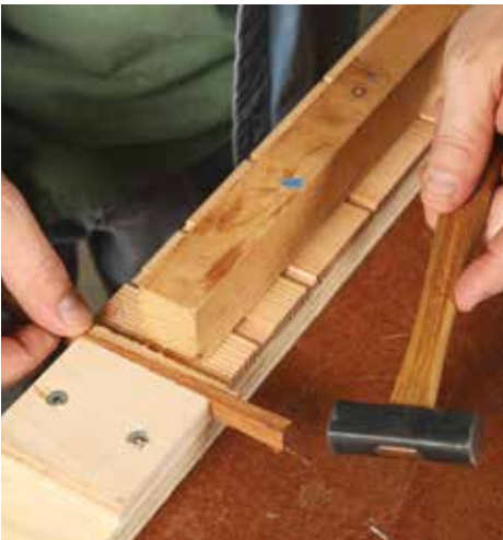
Help from a clamping jig. To simplify assembling the many small panel parts and splines into one wide panel, do the glue-up on a piece of plywood long enough to accommodate all the pieces plus a stop block, two opposing wedges, and a little extra space for the wedges to do their magic.
