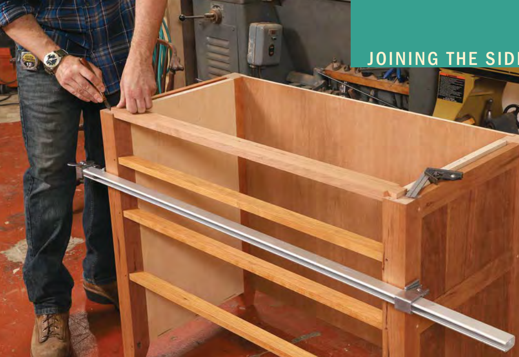
The last link. In order to transfer the top stretcher's dovetail onto the top of the leg, Hill first dry-fits the drawer dividers and the cabinet's back. After tracing the dovetail, he begins the sockets with a trim router, cutting close to his layout lines, and follows up with chisels.
