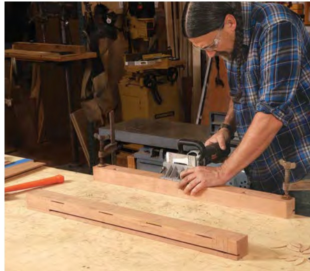
Cutting the slots. After disassembling the side unit, Hill cuts biscuit slots in the plywood panel and the legs. He adds a layer or two of tape to the plywood so that after glue-up the legs will be just slightly proud of the plywood.
