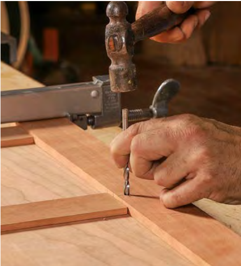
Marking for pins and biscuits. With holes for drawbore pins already drilled in the leg, a tap of the brad-point bit (above left) produces a center mark. After disassembly, Hill will offset the centerpoint mark toward the shoulder slightly so driving the pin will draw the joint tight. To mark for biscuits (above right), Hill clamps the side of the plywood inner case between the legs.
