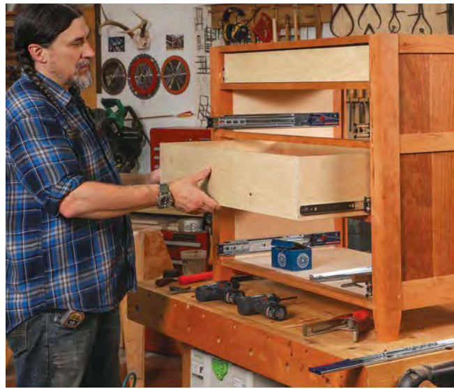
Hanging drawers. The plywood inner case presents a perfect surface for hanging mechanical drawer slides. To simplify hanging them, Hill rests the slide on a spacer clamped to the case side as he drives the screws. He'll use the same spacer to hang the mating slide on the opposite side, and then he'll cut the spacer down to the appropriate height for the next slides.
