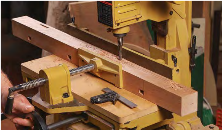
All the mortises. At his hollow-chisel mortiser, Hill chops mortises in the leg for the drawer dividers and then for the rails.
