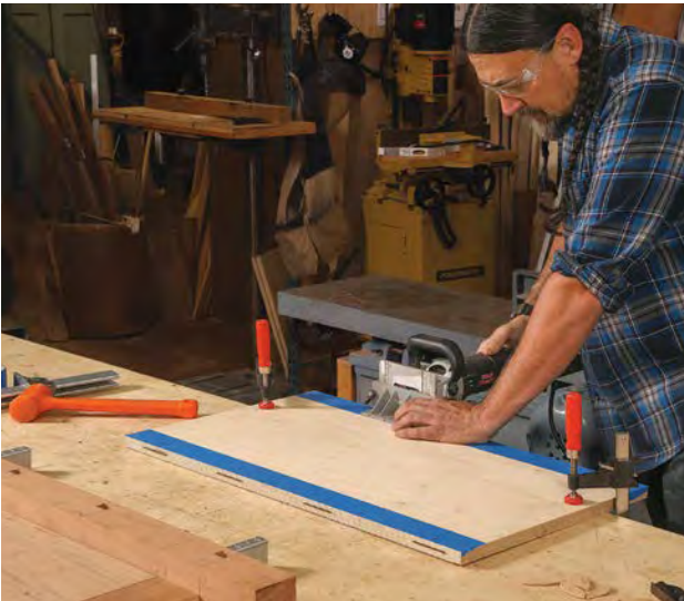
Marking for pins and biscuits. With holes for drawbore pins already drilled in the leg, a tap of the brad-point bit (above left) produces a center mark. After disassembly, Hill will offset the centerpoint mark toward the shoulder slightly so driving the pin will draw the joint tight. To mark for biscuits (above right), Hill clamps the side of the plywood inner case between the legs.
