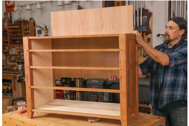
Can't rack with the back. Before the glue sets, Hill slides the back in place dry to help ensure the case is square.
