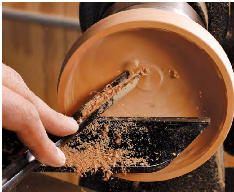
Open up the inside. With a \frac{1}{2} -in. deep-fluted gouge, make a series of progressively wider and deeper hollowing passes toward the center depth hole.
