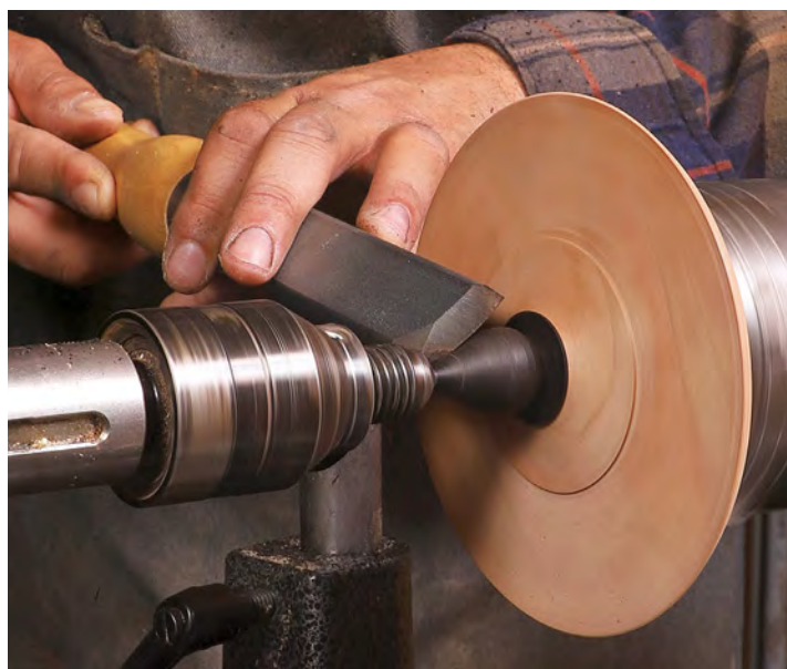
Forming the finial. To turn the finial to a teardrop shape, Monaco uses a skew chisel and a \frac{3}{4} -in. spindle gouge. He does the delicate work with the tailstock snugged up to support the finial's tip.
