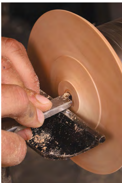
Glue in the finial blank. After turning an ebony finial blank with a tenon to fit the mortise in the lid, Monaco secures it with CA glue.
