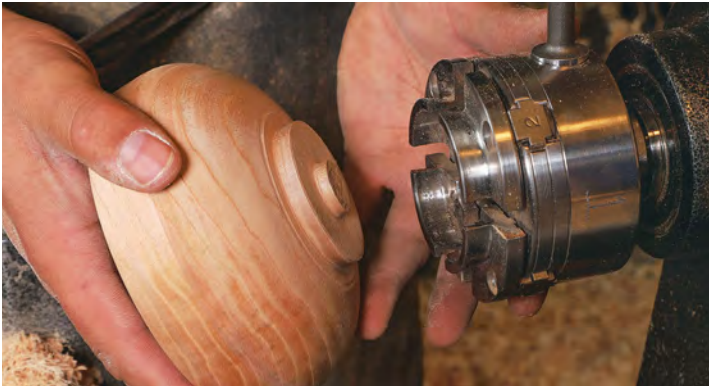
Remount and ream out. After backing off the tailstock, Monaco reverses the blank and mounts the tenon in a four-jaw chuck. With the lathe running slowly, he drills a depth hole, using blue tape around the bit as a depth stop.
