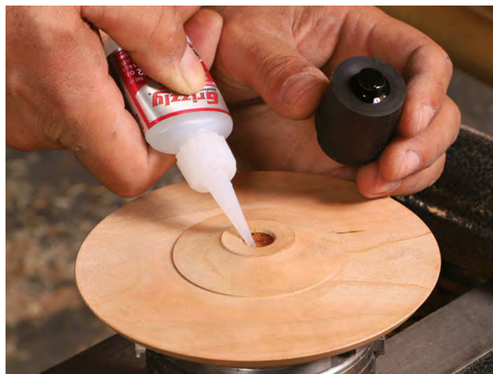
Glue in the finial blank. After turning an ebony finial blank with a tenon to fit the mortise in the lid, Monaco secures it with CA glue.
