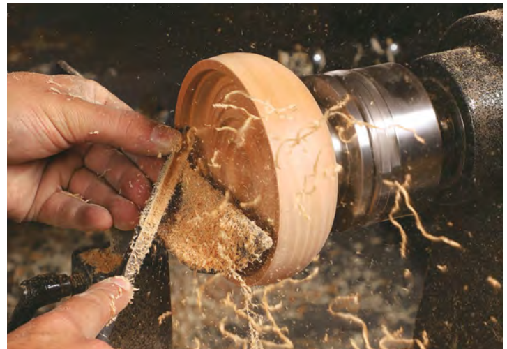
Work the walls. Using bevel-rubbing push cuts with \frac{1}{4} -in. and \frac{3}{8} -in. deep-fluted gouges, Monaco establishes the vessel's final wall thickness.
