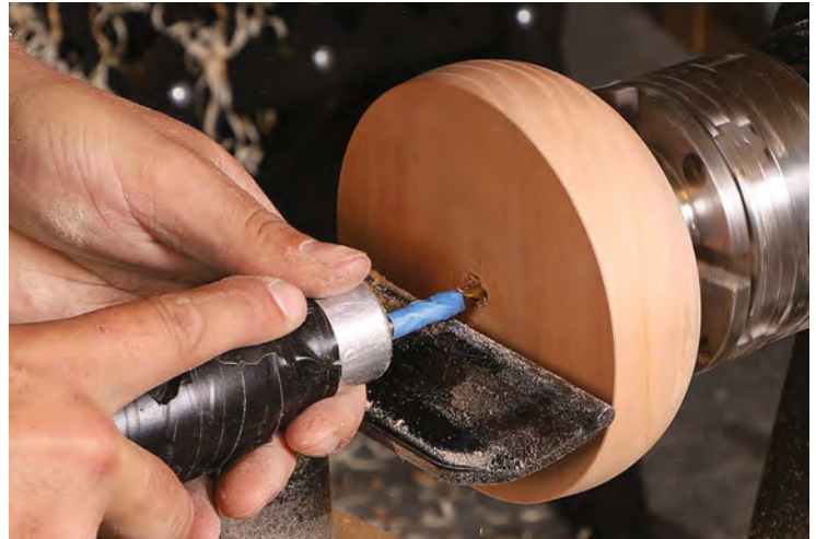
Remount and ream out. After backing off the tailstock, Monaco reverses the blank and mounts the tenon in a four-jaw chuck. With the lathe running slowly, he drills a depth hole, using blue tape around the bit as a depth stop.
