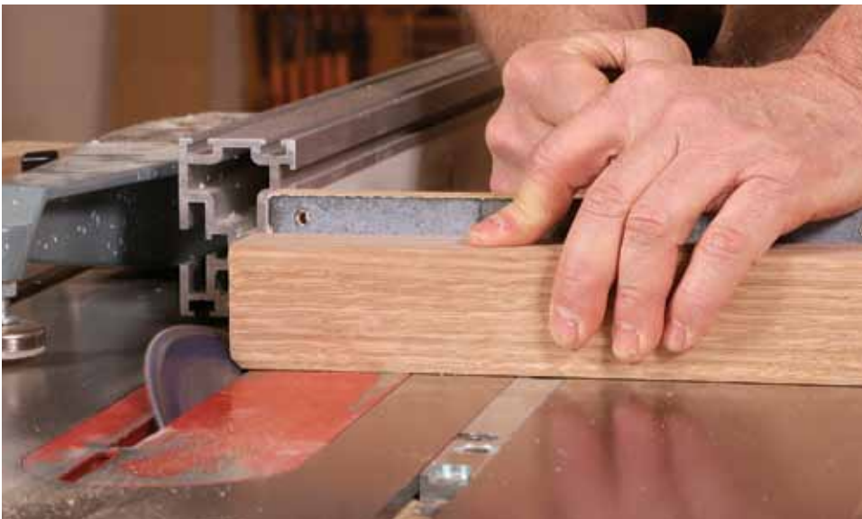
Matching the miter. Using a scrap milled to the width and thickness of the rail, Gochnour sets up the tablesaw to miter the rails.
