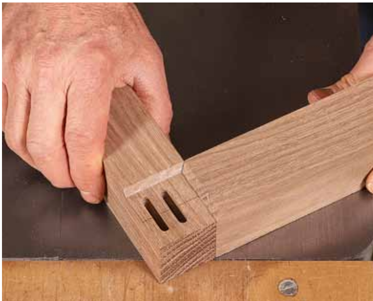
Matching the miter. Using a scrap milled to the width and thickness of the rail, Gochnour sets up the tablesaw to miter the rails.
