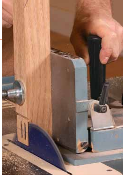
A slice off the inside. The leg surfaces that get the miter also get a shallow recess to accept the rail. Gochnour makes the cut at the tablesaw with a tenoning jig.
