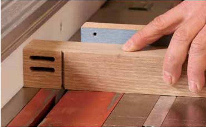
Mini miters. The legs and rails of the base meet in a Barnsley joint—a small miter that divides a shared curve. After cutting Domino mortises, Gochnour cuts the small miters on the two inside faces of the leg.
