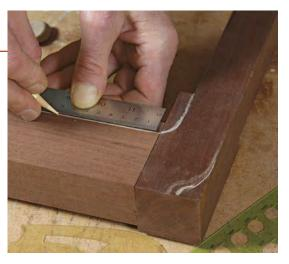
outside faces. With the piece dry-fitted and standing, use tape or a marker to define shapes on the leg or apron. You can do the shaping now, or after assembly.
