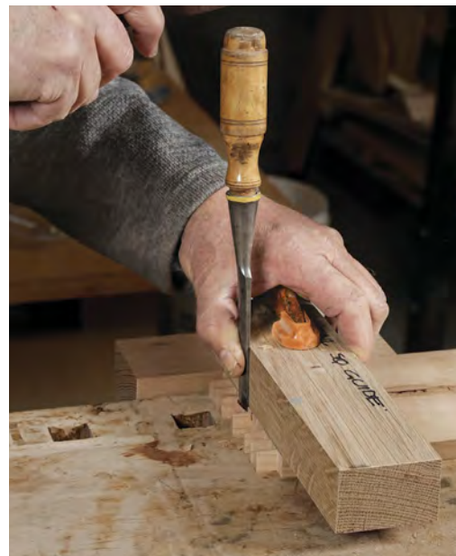
Trim between the pins. Fortune uses his chisel guide when paring the baseline. Because he transferred accurately, the cheeks do not need paring.
