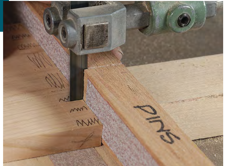
First tilt cuts right side. Cut to the baseline scribed on a scrap, and then clamp the stop against the jig's leading edge. Cut the right side of all the pins on one board, then work through the other pin boards.
