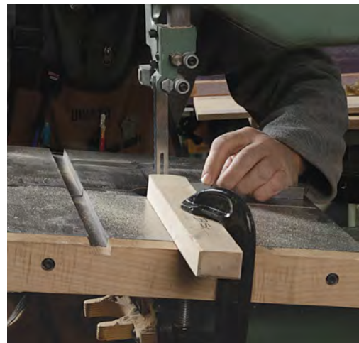
First tilt cuts right side. Cut to the baseline scribed on a scrap, and then clamp the stop against the jig's leading edge. Cut the right side of all the pins on one board, then work through the other pin boards.
