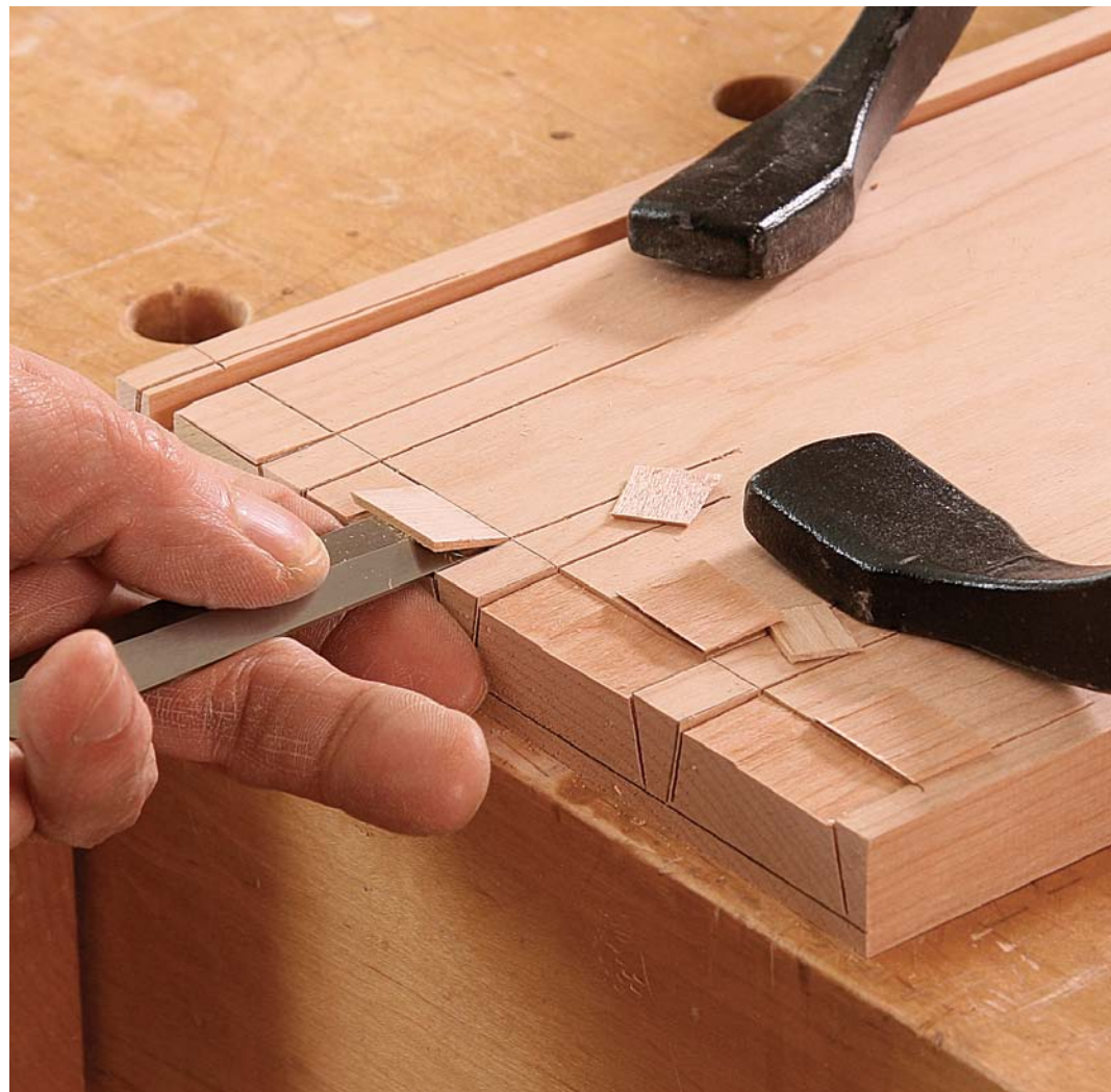
Careful kerfing. With the drawer front at 45° in the vise, saw along the cheeks of the pins until you reach the two scribed lines.
