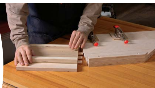
Easy on, easy off. The guide base connects to the clamping base with three dry-fitted Domino slip tenons.
