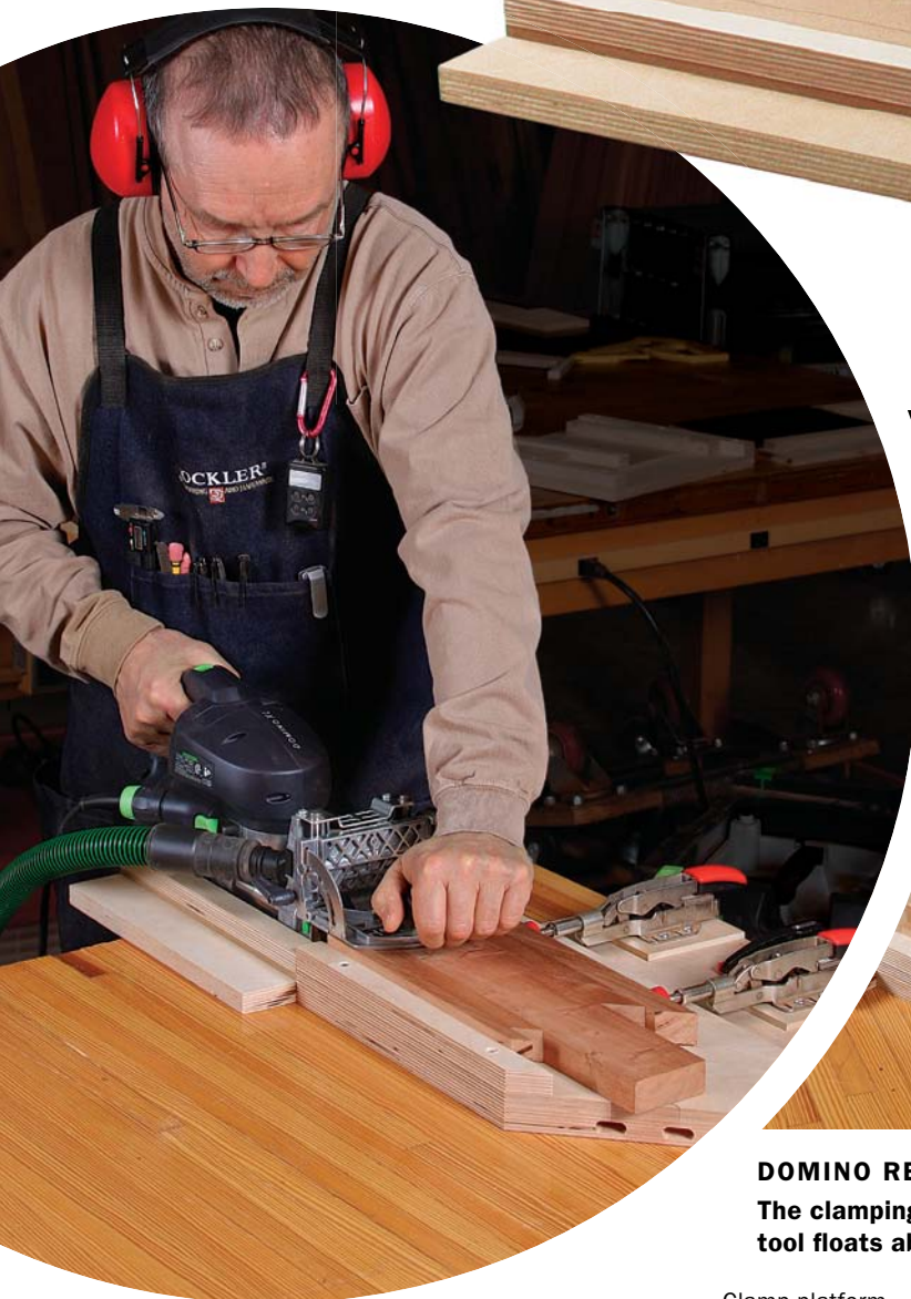
Guide base attaches to left end of clamping base for 90° joints.
