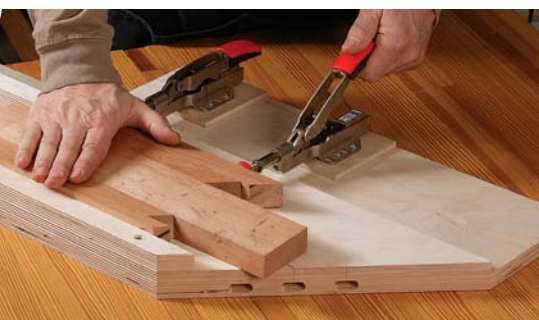
Clamp the workpiece. Add spacer blocks the same thickness as the workpiece, to align the joint's centerline with the jig's centerline.
