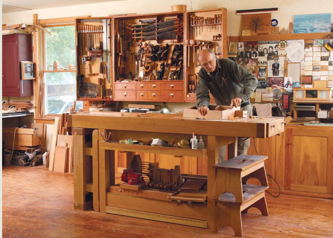
Hand tools within easy reach. One corner of Becksvoort's shop is dedicated to benchwork. His custom-height bench is located near his wall-mounted tool cabinet. And counter-height cabinets along the wall provide ample storage for handheld power tools.
