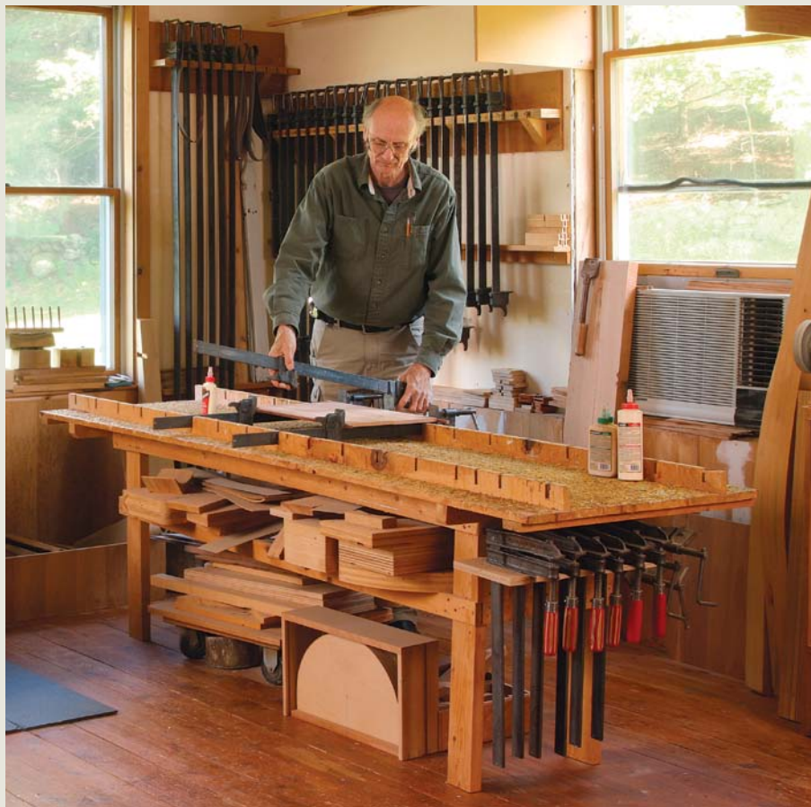
A corner for glue-ups. Becksvoort’s solid-cherry Shaker furniture usually starts with glued-up panels, so a dedicated clamping table is a worthwhile investment in floor space. He assembles doors there, too.
