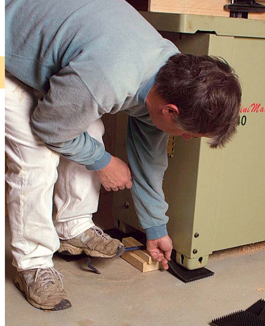
A rubber doormat sliced into small pads and placed under the feet of a machine can significantly reduce the vibration transferred from the shop floor to the framing in the rest of the house.
