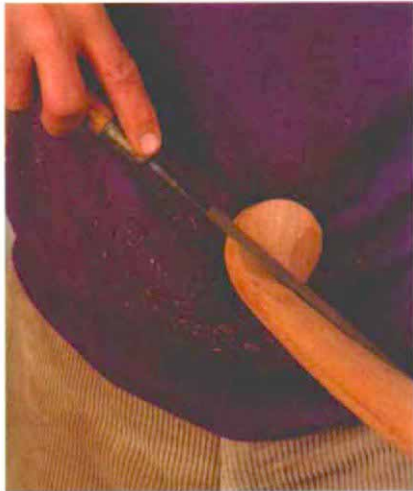
Rasp teeth (above) are formed individually when the steel blank is struck by a punch. The tooth and gullet are formed simultaneously. The two best rasps sold today are the Nicholson #49 and #50. The #49 (right) removes a lot of wood quickly. The #50 leaves a smoother surface.
