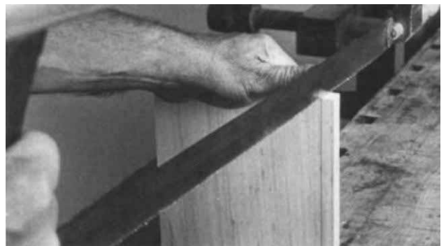
Starting the cut: Frid holds saw loosely, left thumb guiding blade, with eye, blade and cutting line all aligned vertically. Blade is angled so frame will clear wood as cut proceeds.
