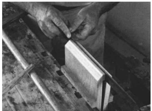
To level the teeth, a mill file is run the length of the blade.
