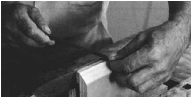
With fingers as stops, whole length of file is used on each stroke.
