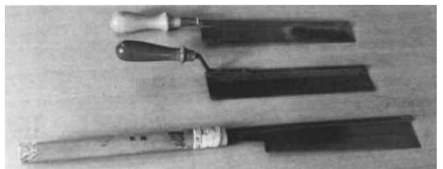
Dovetail saws: straight (top), offset and Japanese.
