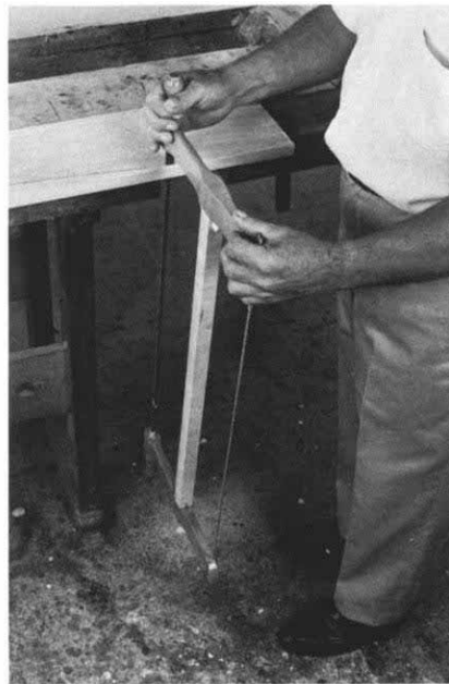
When ripping (left), left hand guides cut and right hand powers whole length of blade downward. Scroll bowsaw (center) also cuts on
